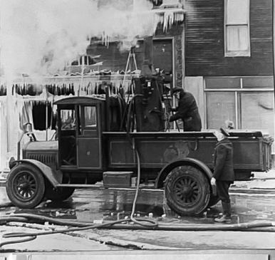
FORMERLY HOSE THAWING DEVICE NO. 1 1918 MACK (JIM O'NEIL) GAINLEY COLLECTION
