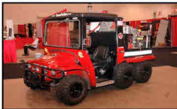
Gator - Fire Special Operations 3950 S Honore St AFFF Foam - 10 gals. 60 gal. Booster tank 50' Hard line hose Ansul
