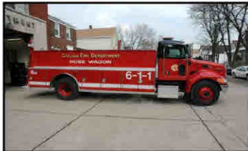
611 Hose Wagon E81 - 10458 S Hoxie Ave Carries 5200 feet of 5 inch hose
